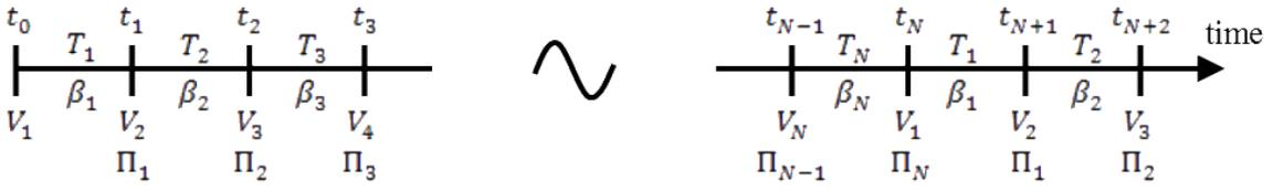
Figure 1: Interval index reference for periodic problems. Note that the return ( $\Pi_k$ ) is yielded at the end of interval  $k$ , but that  $V_k$  refers to the beginning of interval  $k$ .
